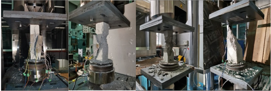
Fig. 2. General view of the failure of test specimens of concrete of different classes.
